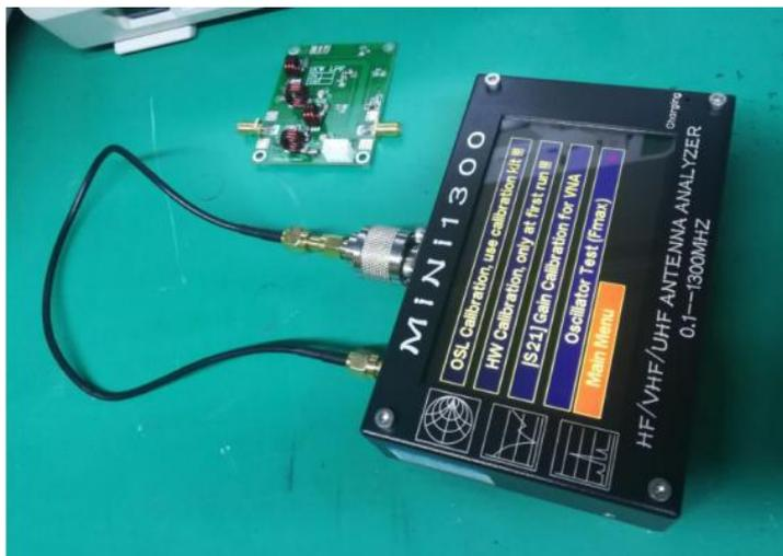
2. Open the Calibration Menu. (S21)Gain Calibration for VNA.
