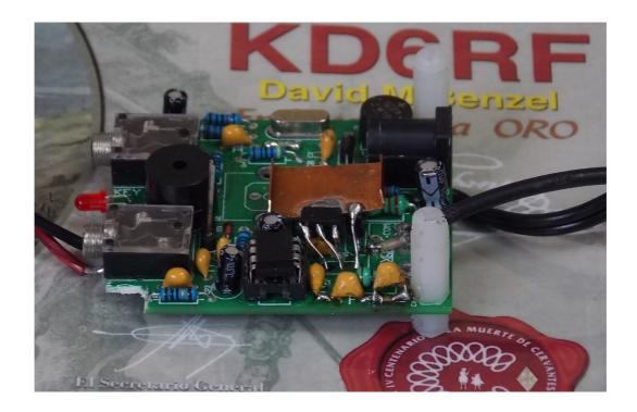
Parallel in the new 150 pF capacitor across the pi-network output capacitor, and that's it for this mod.
